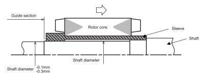
It is recommended that a push-in guide 0.1 to 0.3mm smaller than the outer diameter of the rotor fixing part be created on the shaft.
