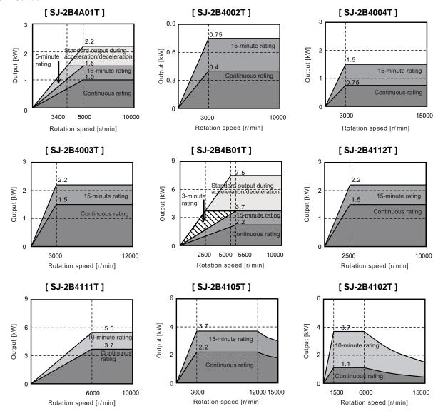
(Note) Actual acceleration/deceleration output is 1.2-fold of "Standard output during acceleration/deceleration" or "Short time rated output".
