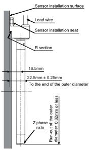
Installing the detector
