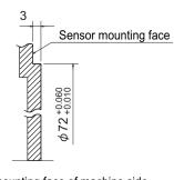
Encoder mounting face of machine side
