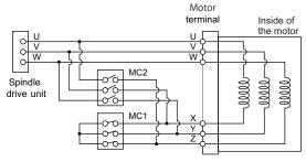
MC1: Contactor to connect low-speed coil ( $\blacktriangle$ -connection) MC2: Contactor to connect high-speed coil ( $\Delta$ -connection)
