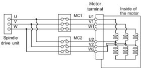
MC1: Contactor to connect low-speed coil (1st ♣ -connection) MC2: Contactor to connect high-speed coil (2nd ♣-connection)
