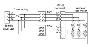
MC1: Contactor to connect low-speed coil (1st **ل**-connection) MC2: Contactor to connect high-speed coil (2nd **ل**-connection)
