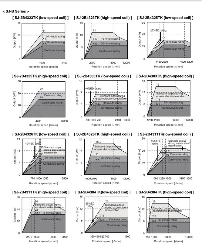
(Note) Actual acceleration/deceleration output is 1.2-fold of "Standard output during acceleration/deceleration" or "Short time rated output".
