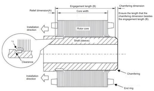
The inside of the rotor is swollen like \*1 as the rotor core is made of layered steel. Therefore, take into consideration the swell in the rotor and ensure the relief dimension (A) and engagement length (B). The following are the relief dimension (A) and engagement length (B).
