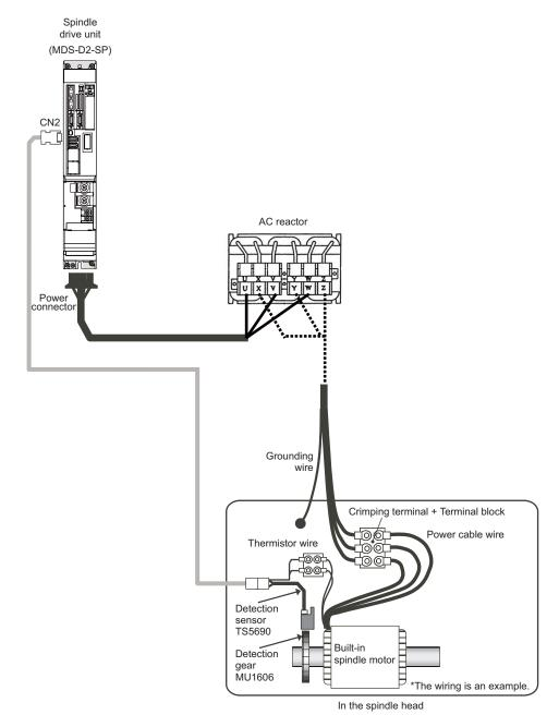
There are no limits to the cable length between the drive unit and AC reactor, and between the AC reactor and built-in spindle motor.
