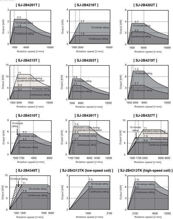
(Note) Actual acceleration/deceleration output is 1.2-fold of "Standard output during acceleration/deceleration" or "Short time rated output".
