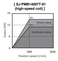
(Note) Actual acceleration/deceleration output is 1.2-fold of "Standard output during acceleration/deceleration" or "Short time rated output".
