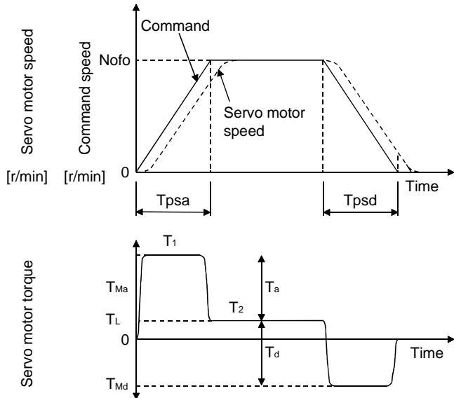
$$T_1 = T_{Ma} + T_L \dots \quad (11-5)$$
