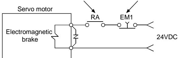
2. The electromagnetic brake is designed for holding and should not be used for ordinary braking.
