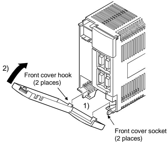
1) Insert the front cover hooks into the front cover sockets of the servo amplifier.
