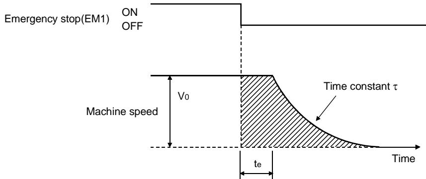
Fig. 9-4 Dynamic Brake Operation Diagram
