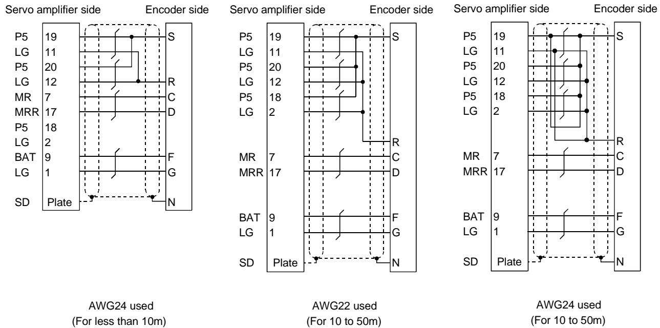
In addition to the above, the customer may also fabricate the cable of the following length:
