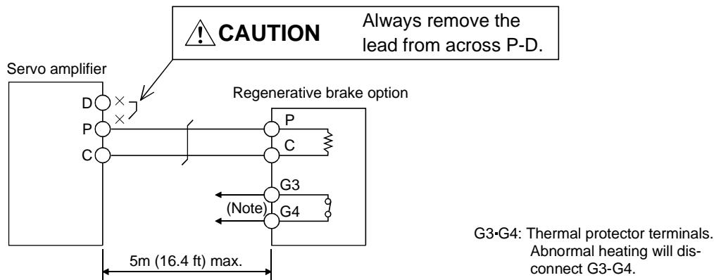
Note: Make up a sequence which will switch off the magnetic contactor (MC) when abnormal heating occurs.
