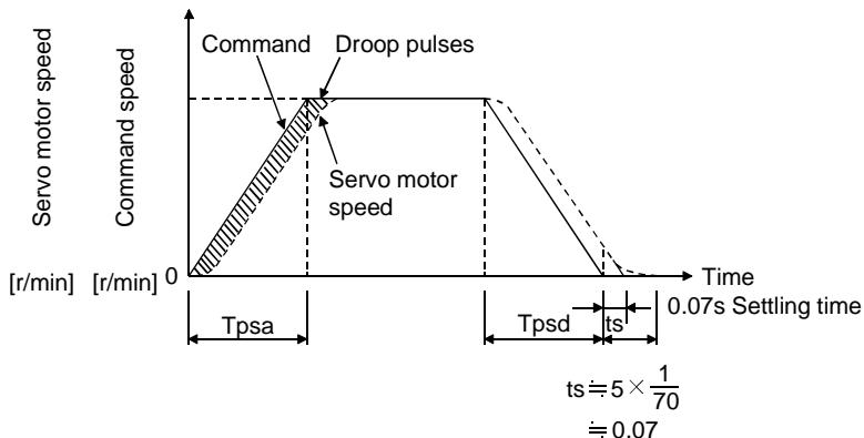
(2) Settling time (ts) during linear acceleration/deceleration
