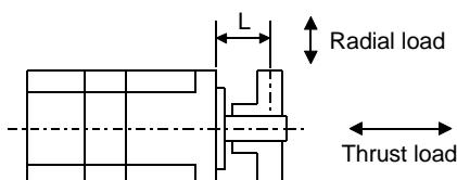
L: Distance from flange mounting surface to load center
