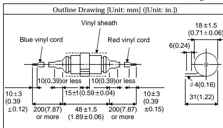
Note that a diode should be installed to a DC relay, DC valve or the like.
