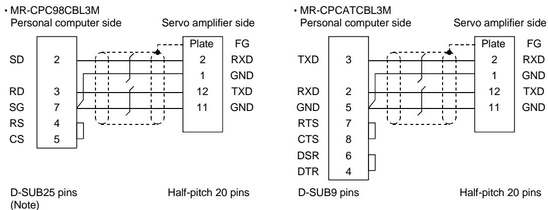
Note: The PC98 Notes having the connector of half-pitch 14 pins are also available. Confirm the shape of the RS-232C connector of the personal computer used.
