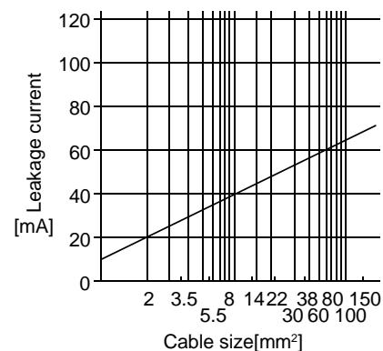
Fig. 6-1 Leakage Current Example
