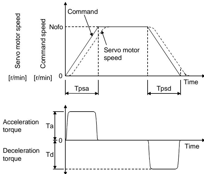
$$\cdot \text{Acceleration torque } T_a = \frac{(J_L+J_M) \cdot N_o}{9.55 \times 10^4} \cdot \frac{1}{T_{psa}} \quad \dots \quad (11-3)$$
